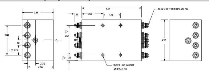
See KK-0851-15 & 25 for standard Mounting Configuration on 15 & 25 Amp Filters
