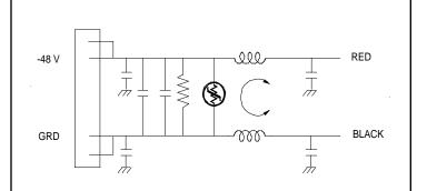
This filter is designed to operate in high current applications of 48 Vdc telecommunication systems. The filter has excellent insertion loss for the small size and also has a varistor for transient protection on the line side. For additional transint protection another varistor can be connected across the load terminals.
