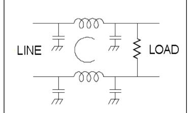
Operating Voltage = \_\_\_\_\_\_48 Vdc Operating Current = \_\_\_\_\_50 Amps
