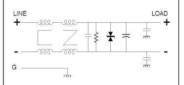
The 1135 series is designed to provide filtering for DC systems operating in very noisy environments.
